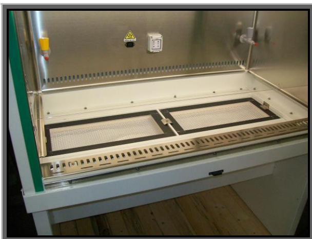
Third hepa filter placed under the work plan
