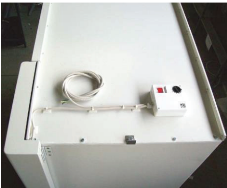
Switch and speed regulator for additional exhaust fan, positioned on the cabinet roof
